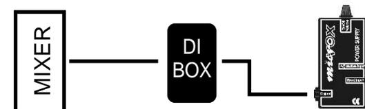
With the M405/M410/M420 systems the PSU has two inputs. Both inputs are factory set at maximum gain. The adjustable input can be turned down in order to balance the mics. See above diagram. Usually, the bass mic is too loud so connect that one to the adjustable input where it can be turned down. The microphone will work with most guitar wireless systems. Plug the guitar transmitter cable into the output socket.
